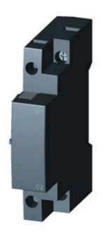
VOLTAGE RELEASE, AC 20...24V, 50/60HZ, 100% ED, AC 20...70V, 50/60HZ, 5SEC ED, DC 20...70V, 5SEC ED, W. SCREW CONNECTION; FOR CIRCUIT-BREAKERS, SZ S00/S0
