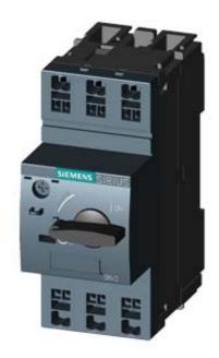
CIRCUIT-BREAKER SZ S00, FOR MOTOR PROTECTION, CLASS 10, A-RELEASE 7...10A, N-RELEASE 130A, SPRING-L. CONNECTION, STANDARD SW. CAPACITY
