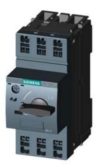
CIRCUIT-BREAKER SZ S00, FOR MOTOR PROTECTION, CLASS 10, A-REL.1.1...1.6A, N-RELEASE 21A, SPRING-L. CONNECTION STANDARD SW. CAPACITY
