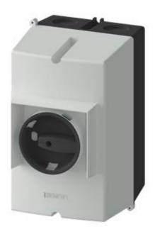
CAST-ALUMINIUM HOUSING IP 65, MOUNTING WIDTH 72MM, WITH PE-TERMINAL FOR CIRCUIT-BREAKERS, SIZE S0
