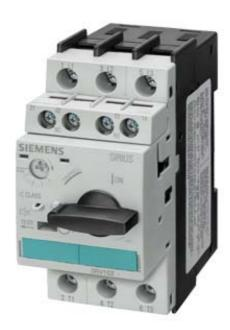
CIRCUIT-BREAKER, SIZE S0, FOR MOTOR PROTECTION, CLASS 10, A REL.17...22 A, N REL.286 A, SCREW CONNECTION, STANDARD BREAKING CAPACITY
