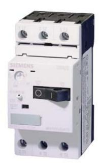
CIRCUIT-BREAKER SIZE S00, FOR MOTOR PROTECTION, CLASS 10, A-REL. 3.5...5A, N-REL. 65A, SCREW TERMINAL, STANDARD SWITCHING CAPACITY
