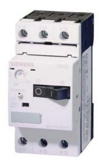
CIRCUIT-BREAKER SIZE S00, FOR MOTOR PROTECTION, CLASS 10, A-REL.2.2...3.2A, N-REL. 42A, SCREW TERMINAL, STANDARD SWITCHING CAPACITY
