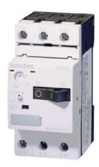
CIRCUIT-BREAKER SIZE S00, FOR MOTOR PROTECTION, CLASS 10, A-REL.1.1...1.6A, N-REL. 21A, SCREW TERMINAL, STANDARD SWITCHING CAPACITY
