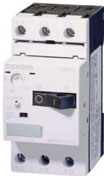
CIRCUIT-BREAKER 0.18...0,25 N-RELEASE 3,3A, SIZE S00, MOTOR PROTECTION, CLASS 10, SCREW CONNECTION STANDARD BREAKING CAPACITY
