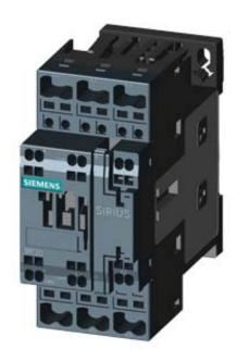
CONTACTOR, AC-3, 7.5KW/400V, 1NO+1NC, AC 230V 50HZ, 3-POLE, SZ SO SPRING-LOADED TERMINAL
