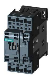
CONTACTOR, AC-3, 5.5KW/400V, 1NO+1NC, AC110V 50HZ, 3-POLE, SZ SO SPRING-LOADED TERMINAL
