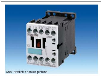
CONTACTOR, AC-3 5.5 KW/400 V, 1 NC, AC 110 V, 50/60 HZ, 3-POLE, SIZE S00, SCREW CONNECTION
