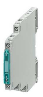
INTERFACE CONVERTER AC/DC 24 V, 2 WAY SEPARATION ON: 0 TO 20 MA OFF: 0 TO 10 V SCREW CONNECTION
