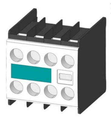
AUXILIARY SWITCH BLOCK, 02, 2NC, DIN EN50005, SCREW CONNECTION, F. CONTACTOR RELAYS A. CONTACT. FOR SWITCHING MOTORS, SIZE S00
