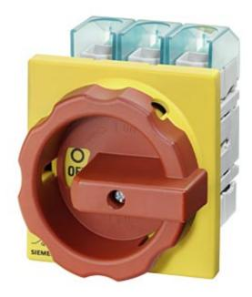
MAIN/EMERG. STOP SWITCH 3-POLE IU=125, P/AC-23A AT 400V=45KW FRONT MOUNTING FOUR-HOLE MOUNTING ROTARY ACTUATOR RED/YELLOW (EMERG. STOP)
