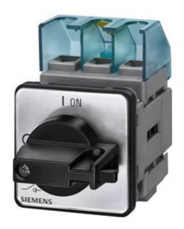
3-P. MAIN CTR./EM.-STOP SWITCH IU=16, P/AC-23A AT 400V=7.5KW FRONT MOUNTING 4-HOLE MOUNTING KNOB-OP. MECH. BLACK
