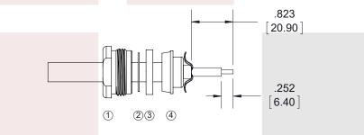
3. SOLDER CONTACT (5) TO CENTER CONDUCTOR. REMOVE EXCESS SOLDER. DO NOT OVER HEAT DIELECTRIC. INSERT CABLE ASSEMBLY INTO BODY (6) & TIGHTEN.
