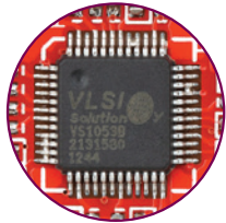
Figure 9-1: On-board VS1053 MP3 codec
