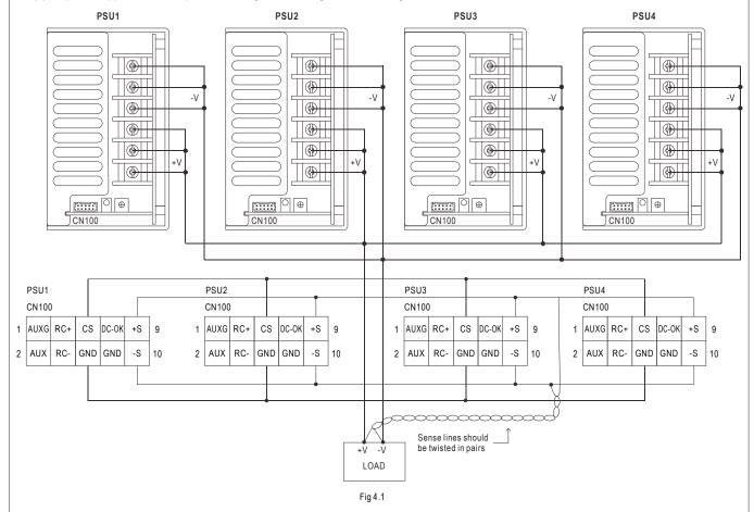
Note: 1.In parallel connection, maybe only one unit (master) operate if the total output load is less than 2% of rated load condition.
