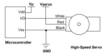
$V\mu$  = microcontroller voltage supply
