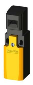
SAFETY POS. SWITCH W. SEPARATE ACTUATOR, PLASTIC ENCLOSURE, 31MM; 1X(M20X1.5) SLOW-ACTION CONTACTS 1NO+1NC, 5 DIRECTIONS OF APPROACH, THE MATCHING SEPARATE ACTUATOR 3SE5000-0AV0. IS TO BE ORDERED SEPARATELY
