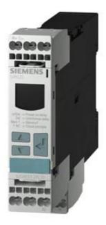
DIGITAL MONITORING RELAY VOLTAGE MONITORING, 22.5MM FROM 17 TO 275V AC/DC OVERSHOOT AND UNDERSHOOT INTERNAL POWER SUPPLY DC AND AC 50 TO 60 HZ SPIKE DELAY 0.1 TO 20S HYSTERESIS 0.1 TO 150V 1 CHANGEOVER CONTACT W. OR W/O ERROR LOG SCREW TERMINAL REPLACEMENT PRODUCT F. 3UG3534, 3UG3535
