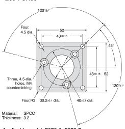
Applicable model: E6C3-A, E6C3-C Note: Three phillips screws M4  $\times$  8 provided
