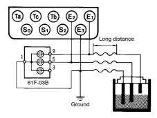
3. When connecting the Surge Suppressor Unit, wire as shown in the following example (with three electrodes).
