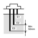
Electrodes are in actual contact with the liquid. Standard electrodes are made of stainless steel and usable in purified water, sea water, sewage, acid (except acetic acid, sulfuric acid, etc.) and alkaline liquids, although they may corrode depending upon the temperature and working conditions.
