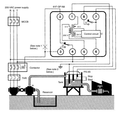
Note: 1. The diagram shows the connections for water supply. When draining, change the connection from terminal 2 to terminal 3.
