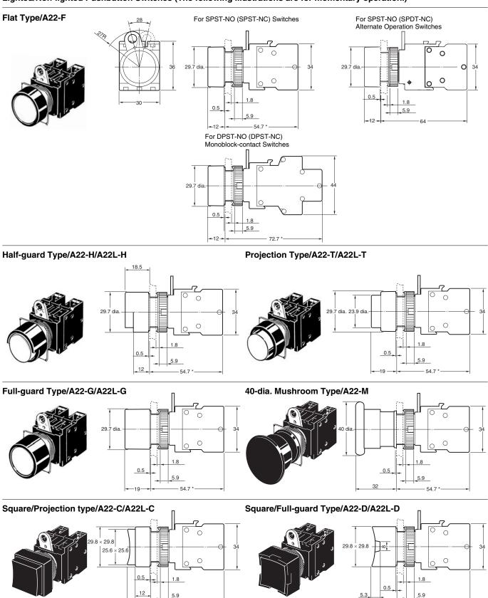
Note: Lighted models have the same dimensions as shown above, whether they are with or without Voltage Reduction Units. \* Alternate operation models are 9.3 mm longer.
