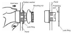
When the panel cutout dimension is 25 dia., remove the supplied rubber washer and mount the 25-dia. Ring as shown below. (Since the A22Z-R25 is not attached to the main body, order separately.)
