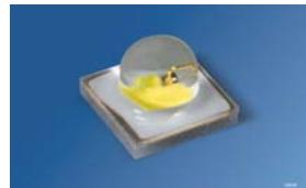
Small size high flux LED for slim designs (between 100 mA and 800 mA constant current). 87 lm (typ.), 80 lm/W (typ.) at 350 mA (3000 K).
