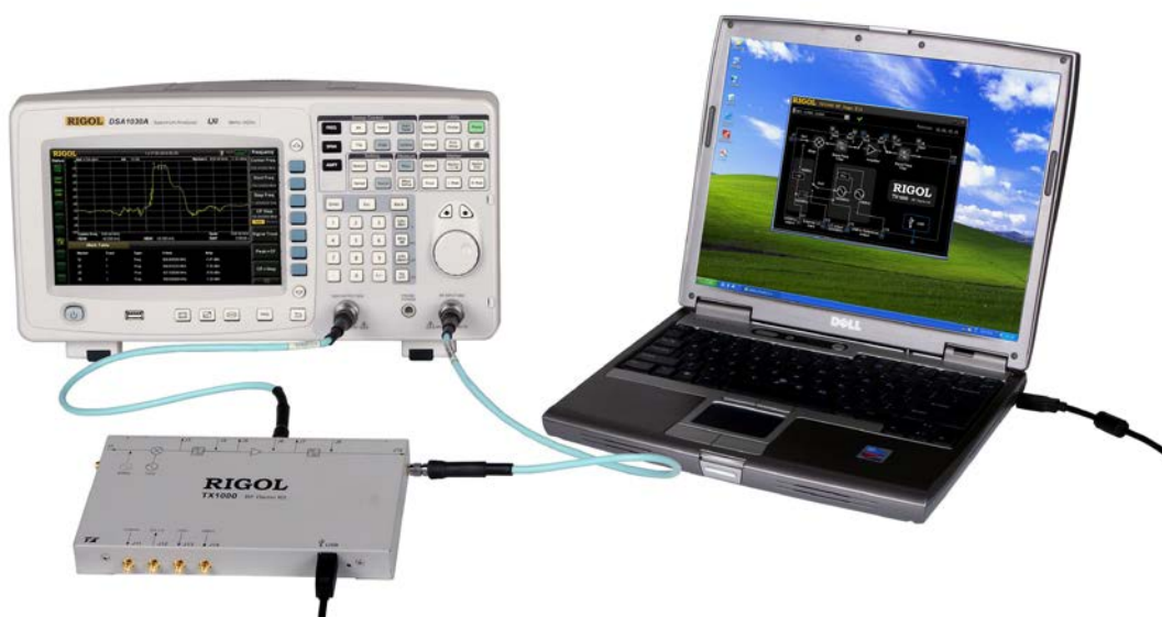
Figure 7 Test the Band-pass Filter Characteristics
