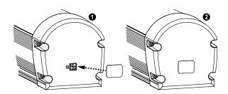
Figure 4. Installing the cascade cover (step 9)
