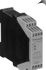
The FF-SRL6025 module is designed to be used with safety devices with safety static outputs when danger to personnel or machinery is present. This safety control module provides an emergency stop signal to the machine control circuitry.
