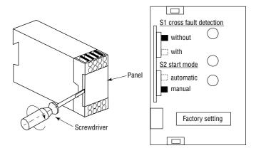
The FF-SRL6025 emergency stop module contains two internal switches (S1 and S2) for the mode settings. To access to these switches, remove the front panel using a screwdriver.
