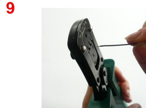
Insert the cable until insulation stop blade!
