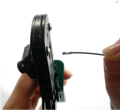
Remove the crimped contact.
