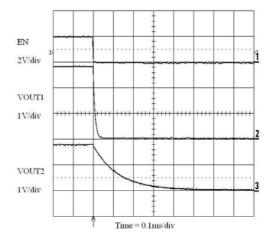
Figure 21. Enable Turn-off (300 mA/100 μA Loads)
