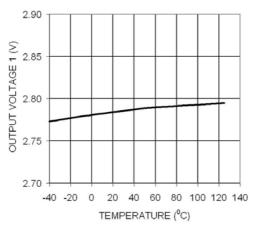
Figure 3. Output Voltage 1 vs. Temperature
