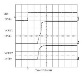
Figure 20. Enable Turn-on (300 mA/100 μA Loads)
