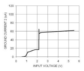
Figure 10. Ground Current (EN1 = GND)
