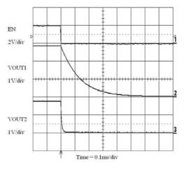
Figure 23. Enable Turn-off (100 μA/300 mA Loads)
