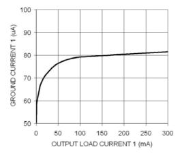
Figure 7. Ground Current (EN2 = GND)
