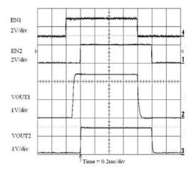
Figure 29. Separate Enable Operation (100 mA Loads)
