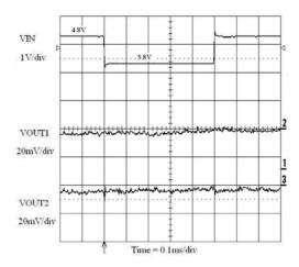
Figure 27. Line Transient Response (0.1/100 mA Loads)
