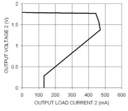
Figure 14. Output Voltage 2 vs. Load Current 2
