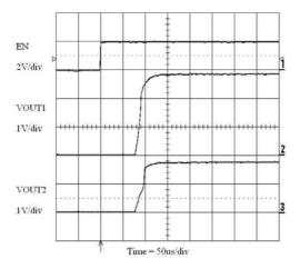
Figure 22. Enable Turn-on (100 μA/300 mA Loads)
