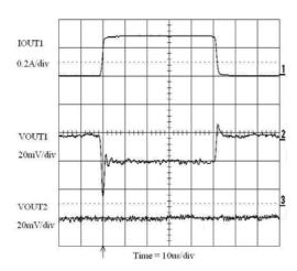
Figure 24. VOUT1 Load Transient Response (0.1 to 300 mA)
