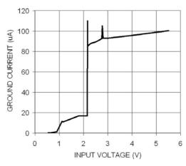
Figure 12. Ground Current vs. Input Voltage
