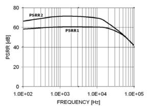
Figure 17. PSRR 1 & 2 vs. Frequency (30 mA Load)
