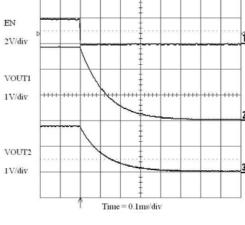
Figure 19. Enable Turn-off (100 μA Loads)
