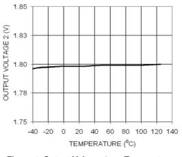
Figure 4. Output Voltage 2 vs. Temperature
