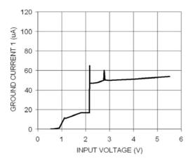
Figure 9. Ground Current (EN2 = GND)
