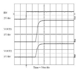
Figure 18. Enable Turn-on (100 μA Loads)
