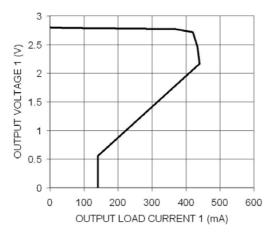
Figure 13. Output Voltage 1 vs. Load Current 1
