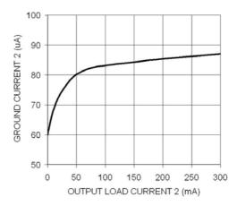
Figure 8. Ground Current (EN1 = GND)
