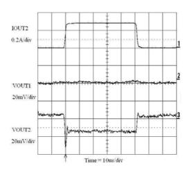
Figure 25. VOUT2 Load Transient Response (0.1 to 300 mA)
