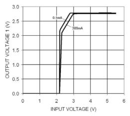
Figure 11. Output 1 Dropout Characteristics
