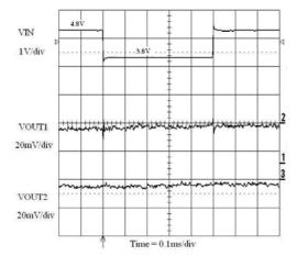
Figure 28. Line Transient Response (100/0.1 mA Loads)
