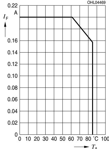
**Zulässige Impulsbelastbarkeit  $I_F = f(t_p)$** **Permissible Pulse Handling Capability**Duty cycle  $D$  = parameter,  $T_A = 25^\circ\text{C}$ **Pulse derating under steady state condition**(conditions: still air; FR4;  $R_{th,JA}$  150 K/W)
