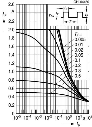
**Zulässige Impulsbelastbarkeit  $I_F = f(t_p)$** **Permissible Pulse Handling Capability**Duty cycle  $D$  = parameter,  $T_A = 70^\circ\text{C}$ **Pulse derating under steady state condition**(conditions: still air; FR4;  $R_{th,JA}$  150 K/W)
