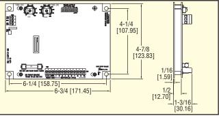
Ideal for pneumatic conveying systems, the Series DCT500ADC Low Cost Timer Controller is designed to provide continuous or on-demand cleaning for 10-35 volt powered receivers and pulse jet systems. Available in either 4, 6 or 10 channels, each unit is the same size, minimizing enclosure space and reducing overall system installation cost.
