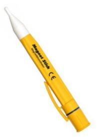
The Magnet Stick is an instrument for testing the presence of magnetic fields. By simply holding the tip of the instrument near the test area, it indicates a magnetic field by glowing. The test lamp responds to all kinds of magnetic fields, from alternating current to direct current and permanent magnets. (Sensitivity 300 gauss 0,3 mT) **General Features:**
