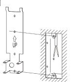
※As shown in the above diagram, the Metal Fitting and wiring can be installed in a junction box (UL listed 3.5/16" pitch or JIS C8336 83.5mm pitch). However, the unit will not be water-tight.
