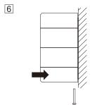
Install and tighten the two screws (M4 x 35) removed in step [1] at the bottom of the lower cover.
