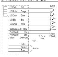
CAUTION Only apply voltage to the Power Supply Wire.
