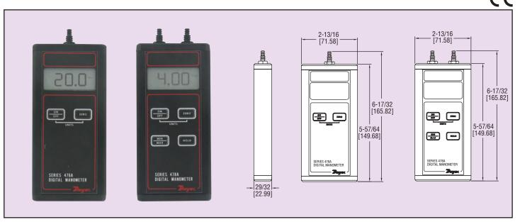
**Ideal for field or laboratory use,** the Model 476A Single Pressure Digital Manometer measures low pressures from -20 to 20 in w.c. with  $\pm 1.5\%$  full scale accuracy. Designed especially for the HVAC contractor, the Model 476A can be used to set supply pressures, verify pressure switch operation, adjust regulators, check pneumatic systems and computer peripherals. The rugged, handheld unit is constructed with an extruded aluminum case for exceptional durability.
