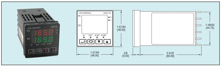
The compact Series 16C Temperature Controller offers accurate temperature measurement and control in a 1/16 DIN package. Designed for direct or reverse acting (cooling or heating) control, the Series 16C can be programmed for simple ON/OFF or more complex PID control functions. PID control is supported with manual or auto-tuning. Select relay, voltage or current output for control methods.
