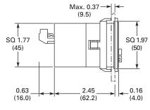
With Front Bezel No. 2 Panel Cut-Out 1.97 x 1.97 (50 x 50)
