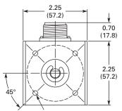
(4) 6.32 (160.5) Tapped Holes 0.25 (6.4) Deep on 2.00 (50.8) B.C. (Same Mtg. Holes on Opposite End and Bottom)
