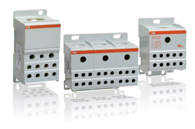
Using a Distribution Block eliminates the need to wire each device in the control circuit back to the power source by using one large wire on the input side, and several smaller wires on the output side to your devices downstream. This will give your electrical panel a clean and professional look.
