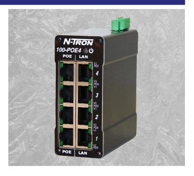
The 100-POE4 automatically detects any PoE device that is connected and powers it accordingly. If a PoE fault is detected on a specific port the Auto-disconnect feature disables PoE power on that port, allowing only data communications to pass. This reduces the risk of damaging costly equipment.
