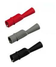
Set of three (one red, one gray, one black) safety designed insulated Probe Tip Alligator Clips. Designed for use with STL 120 Shielded Test Leads and TL75 Test Leads. Accepts standard 0.08" (2mm)-pin tip sized test probes. Nickel-plated steel jaw contact material with standard jaw opening of 5/16" (8mm).
