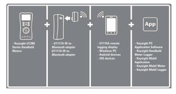
Figure 7. Keysight Remote Link solution
