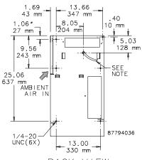
BACK VIEW NOTE: Service cord terminated with appropriate plug cap.
