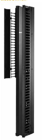
MAXRACK™ Air baffle and Vertical Cable Manager accessory kits ensure CISCO switch compliance. They provide the required cold air access and provisions for high-density cabling. Baffles and cable manager uprights made of aluminum; supporting fingers made of composite. Finish is RAL 9005 black light-textured, low-gloss polyester powder paint.
