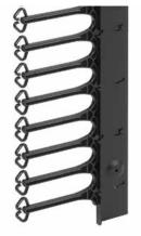
Fingers separate, support and manage cable. Bracket mounts on either left or right side of 700- and 800-mm cabinets between the frame and the rack angle to create vertical wiring space. Bracket has RAL 9005 black polyester powder paint finish. Fingers are molded black plastic. Mounting hardware included. NOTE: Refer to the table to calculate the number of reducing brackets required.
