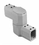
Joint is cast aluminum with RAL 7035 light-gray polyester powder paint finish. Turning range is 360 degrees with stop. Includes access plates for easy wire installation, installation hardware and gasket. Use of the intermediate joint reduces pendant arm load capacity by 43 percent.
