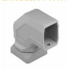
Turning range of 300 degrees. Maintenance-free bearing is steel and polyamide. Includes access plate for easy wire installation. Cast aluminum finished in RAL 7035 light-gray polyester powder paint. Installation hardware, mounting fasteners and gasket included.
