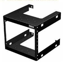
Economical solution for banks of small networking equipment. Integral VELCRO® cable tiedown slots facilitate cable routing. Made of 16 gauge steel, finished with RAL 9005 low gloss black polyester powder paint. Shipped in four easy-to-assemble sections.
