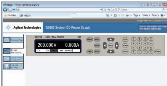
Figure 3. N8900 Series web graphical user interface for remote access and control of the power supply
