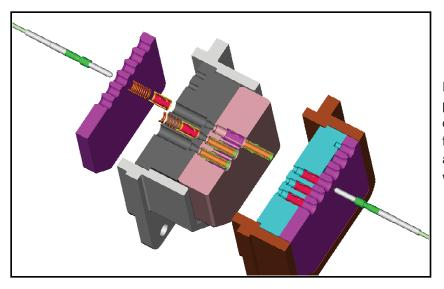
PHD Terminus retention is via Cannon's patented "Little Ceasar" contact retention clip technology. This allows unparalleled flexibility in installing, servicing, cleaning and repairing single optical channels without disturbing parallel channels.
