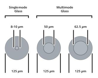
Figure 3. Optical Fiber Sizes
