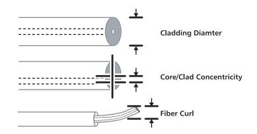
Figure 8. Cladding Diameter, Core/Clad Concentricity, and Fiber Curl
