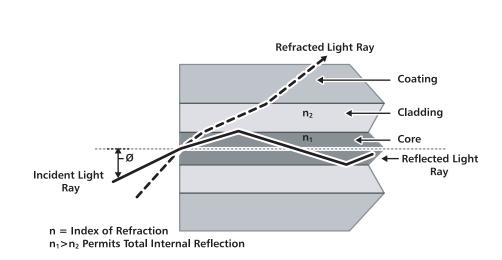
A protective coating is applied to the glass fiber as the final step in the manufacturing process. This coating protects the glass from dust and scratches that can affect fiber strength. This protective coating can be comprised of two layers: a soft inner layer that cushions the fiber and allows the coating to be stripped from the glass mechanically and a harder outer layer that protects the fiber during handling, particularly the cabling, installation, and termination processes.
