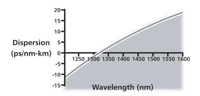
Chromatic dispersion consists of two kinds of dispersion. Material dispersion refers to the pulse spreading caused by the specific composition of the glass. Waveguide dispersion results from the light traveling in both the core and the inner cladding glasses at the same time but at slightly different speeds. The two types can be balanced to produce a wavelength of zero dispersion anywhere within the 1310 nm to 1650 nm operating window.
